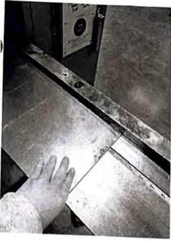
Step 4 - Make sure metal is against the fence
